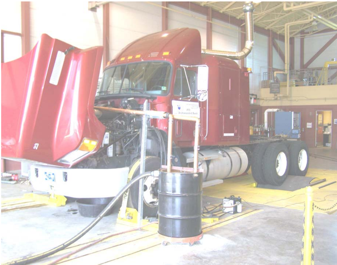
Figure 1: Tractor mounted on the chassis dynamometer with the external cooling system
